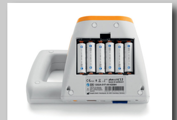
Battery-operated (rechargeable standard AA batteries)
